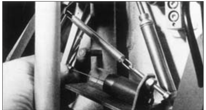
Tension arm damping in a professional video recorder.
