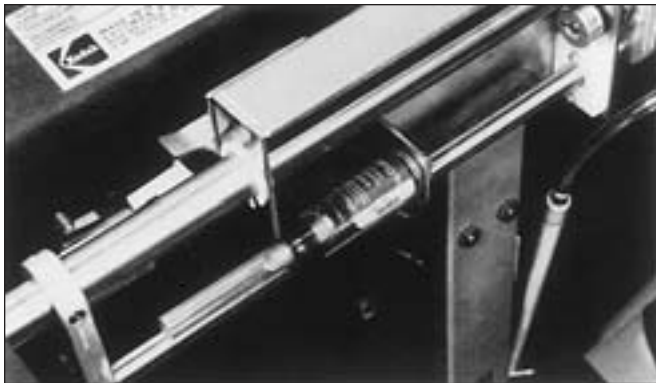
Snubbing paper carrier in an office copier.
