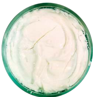
In an oven at 232 °C (448 °F) for 40 hr, Krytox™ lubricant had 0% weight loss.
