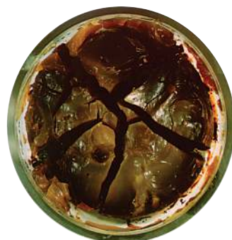
In an oven at 232 °C (448 °F) for 40 hr, the hydrocarbon lubricant had 40% weight loss.
