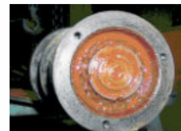
Paper machine bearing: 13 months without topping up.
